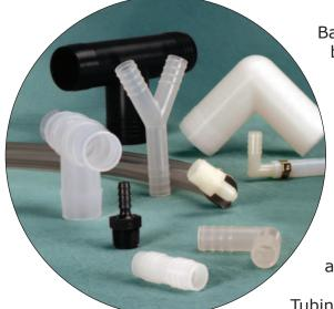
Barbed fittings are usually applied by hand without tools, and typically clamps or cable ties are used to securely attach the fitting to the tubing and ensure a good seal. Sometimes on lower pressure applications, clamps may not be necessary, but that is the exception rather than the rule and should always be determined by testing the connections as they will be used in the actual application.
