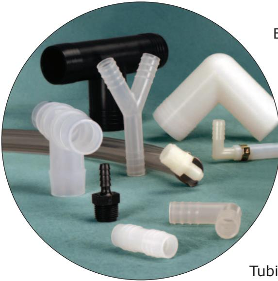
Barbed fittings are usually applied by hand without tools, and typically clamps or cable ties are used to securely attach the fitting to the tubing and ensure a good seal. Sometimes on lower pressure applications, clamps may not be necessary, but that is the exception rather than the rule and should always be determined by testing the connections as they will be used in the actual application.
